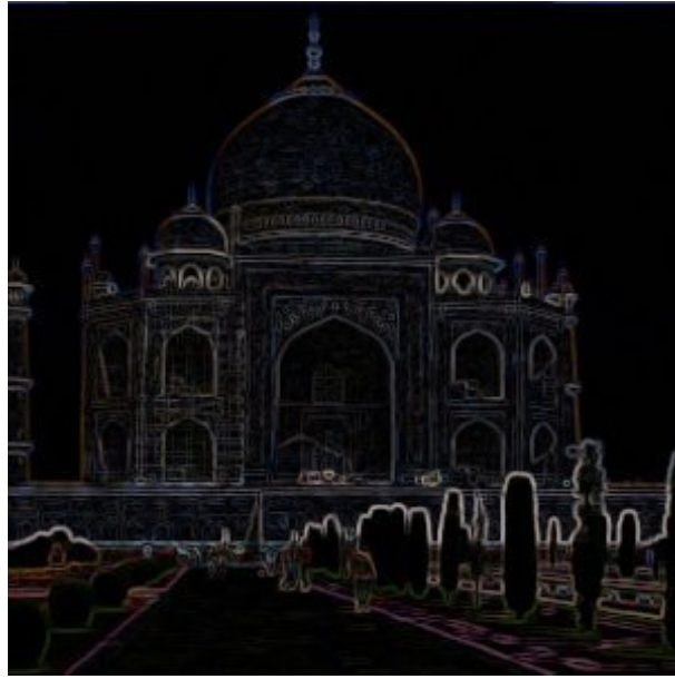
Figure 2: Application of the Sobel filter, highlighting image edges [2].
